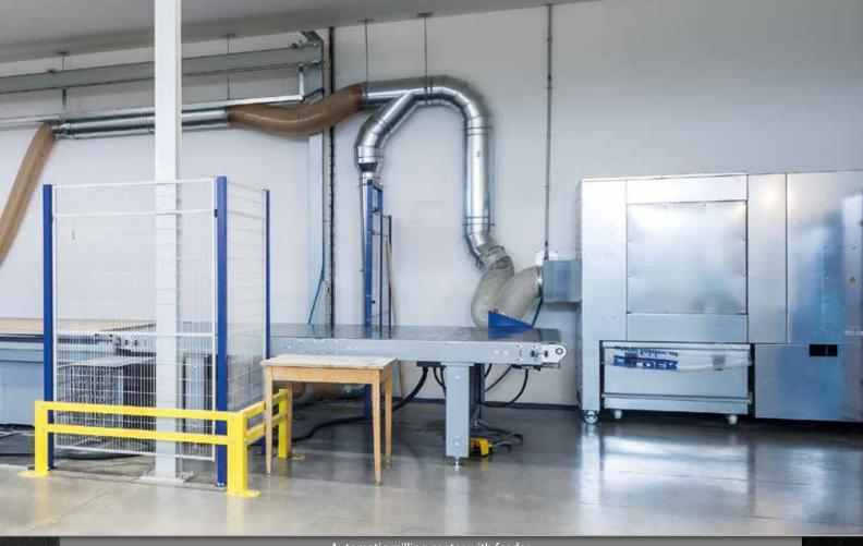
Automatic milling center with feeder
